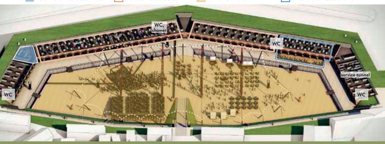
BASTION AREA: 17,000 m<sup>2</sup> ARENA (canopy and entire bastion yard): 9,700m<sup>2</sup> UNDER THE CANOPY: 5,500 m<sup>2</sup> CASEMATE VAULTS: 58 vaults provided with electricity, total area 2,200 m<sup>2</sup>.
